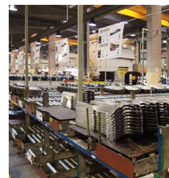
3 7 m roller chute connecting press and welding shops
